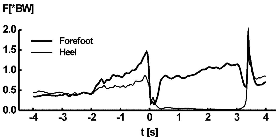
Fig. 6. Mean of the forces at the forefoot and heel over time during hill jumps ( $n = 22$ ,  $t = 0$ : take-off). Reproduced with permission from Schwameder and Müller (1995).
