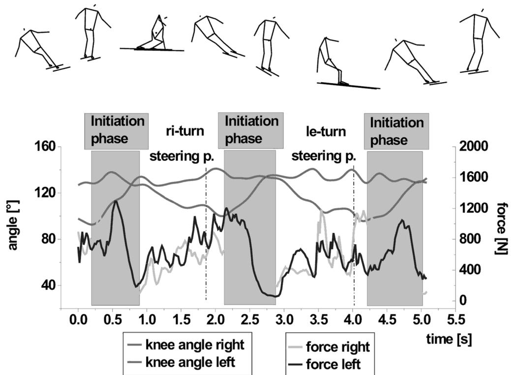
Fig. 4. Ground reaction forces and knee angles during two turns with the carving technique (mean values of six runs). Reproduced with permission from Schiefermüller *et al.* (in press).
