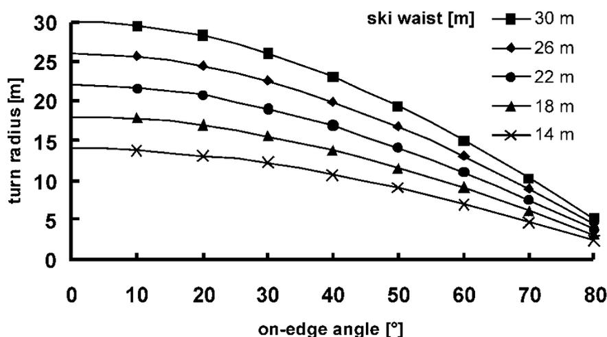
Fig. 2. Turn radius as a function of on-edge angle for variously waisted skis.
