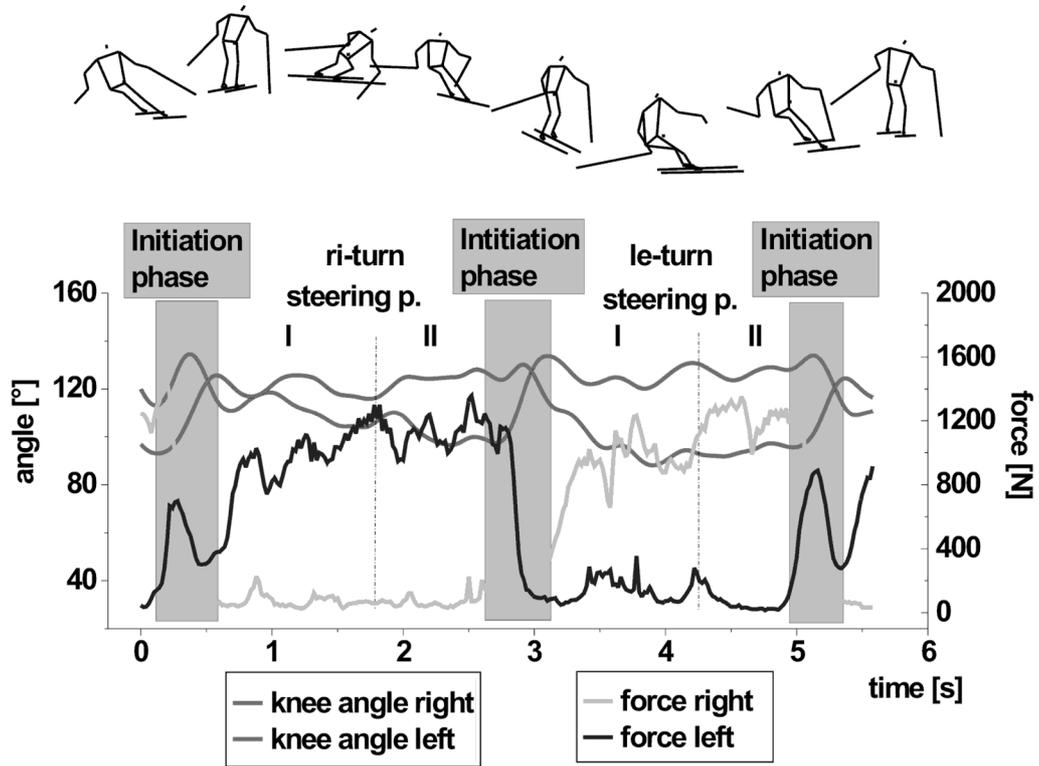
Fig. 3. Ground reaction forces and knee angles during two turns with the traditional parallel technique (mean values of six runs). Reproduced with permission from Schiefermüller *et al.* (in press).
